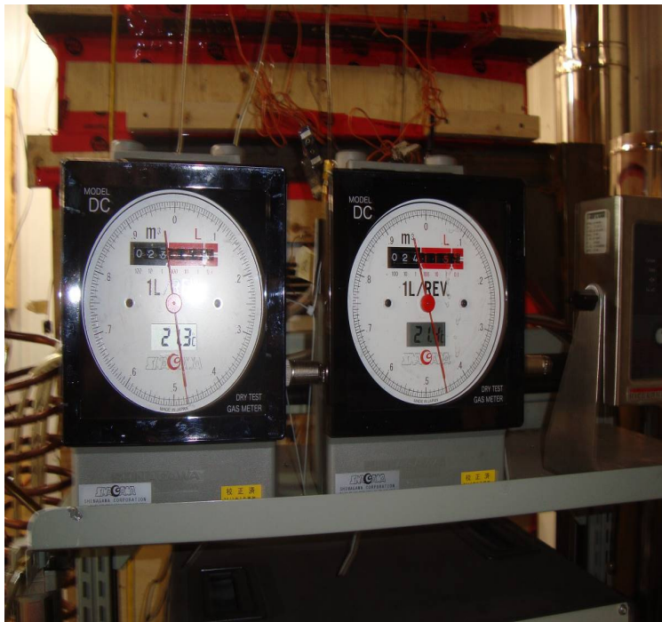
Picture 11 : Dry gas meter
