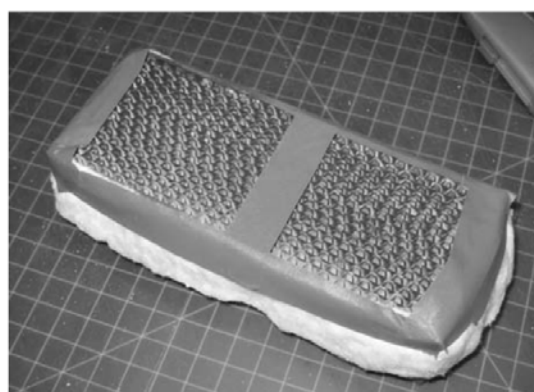
Figure 20 - Installing Gasket on Catalyst
